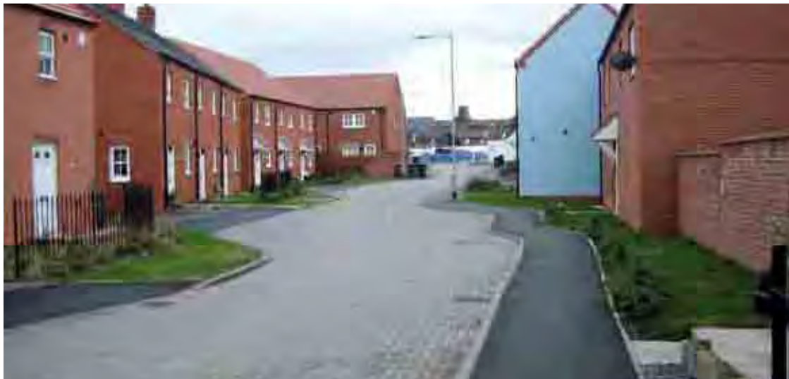
Figure 7.14 This street avoids the use of vertical traffic-calming features, but the irregular alignment is unsightly and unlikely to have much speed-reducing effect, because of the width of the carriageway. It also results in irregular grassed areas that create a maintenance burden while contributing little to street quality.
